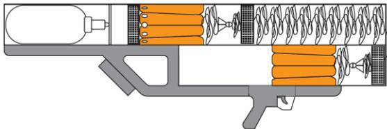
BCB have also designed and make two larger versions. The Buccaneer launcher, (shown here) will fire, also using only compressed air, a det line up to 100 meters. The larger WBS will fire over 300 meters.
