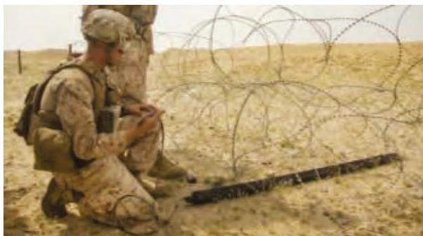
Another innovation available from the BCB range, which will help this dangerous and tedious mine clearance work, is the new ROCK (Rapid Obstacle-Clearing Kit) Stick. Each 2-meter-long rod can be unrolled in seconds and added together to make a longer extension. It can then be triggered
